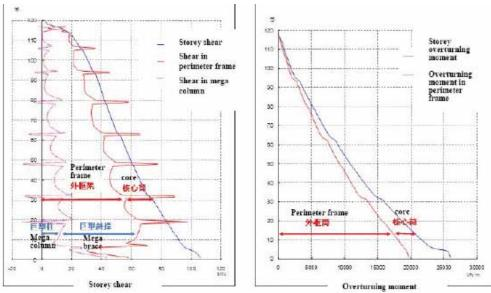
Figure 11. Distribution of shear and overturning moment between internal and external frame 图11. 剪力及倾覆弯矩在内外框架分布示意图
