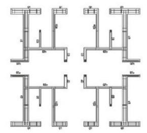
Figure 7. Diagram of composite steel plate shear walls. 图7. 复合钢板剪力墙图表
