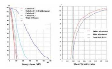
Figure 9. Story shear and frequent earthquake shear-gravity ratio distribution 图9. 楼层剪力和小震剪重比分布图
