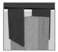
Figure 6. Elevation of perimeter frame and slotted joint at the top 图6. 周边框架立面布置图和顶部滑动连接节点
