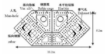
Figure 8. Typical low zone 45m<sup>2</sup> Mega Column section detail 图8. 底部典型楼层巨型角柱45m<sup>2</sup>截面构造示意图
