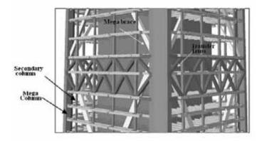
Figure 5. Illustration of Mega Frame and Mega Brace connection – double-story truss
