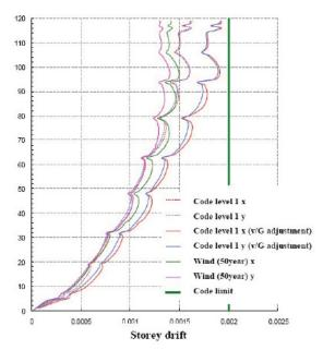
Figure 10. Inter-story drift under earthquake and wind 图10. 地震及风作用下层间位移角
