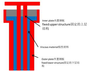
Figure 6. Basic Composition of a Viscous Damper (Source : Obayashi Corporation) 图6. 粘性阻尼器基本组成(出自:大林组)
