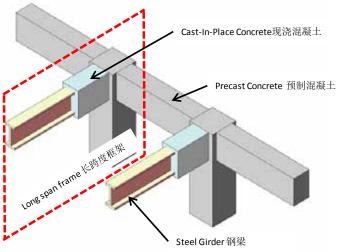
Figure 11. Figure 11: Configuration of a portion scramble steel Girder-Reinforced Concrete (Source:Obayashi Corporation) 图11. 梁-加固混凝土混合结构(来源: 大林组)
