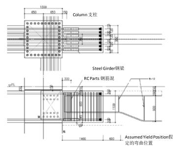
Figure 12. Detailed Drawing RC-S Joint (Source: Obayashi Corporation) 图12. 钢筋混凝土-钢梁接合处详图(来源:大林组)
