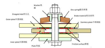
Figure 5. Basic Composition of a Brake Damper (Source: Obayashi Corporation) 图5. 制动片阻尼器基本组成(出自: 大林组)
