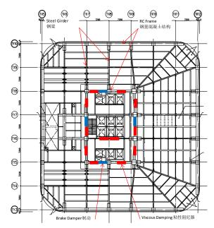
Figure 2. Office Standard Floor Framing Plan (Source: Obayashi Corporation) 图2. 办公室标准层框架平面布置图(出自:大林组)
