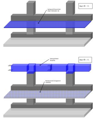
Figure 8. Construction Process (Source:Obayashi Corporation) 图8. 施工过程(出自: 大林组)
