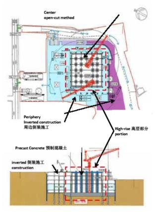
Figure 10. Plan of Temporary Works of Underground Construction (Source: Obayashi Corporation) 图10. 地下建筑临时工程计划(来源:大林组)
