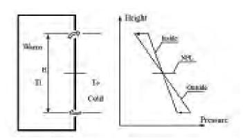
Figure 3. The diagram of air pressure inside and outside of a building vertical space (Source: Jianqiang Li)
