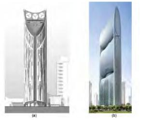
Figure 4. The combination of wind turbine and super tall building (Source: a: Waite, 2009, b: SOM) 图4. 风涡轮与建筑的结合方式 (资料来源: a: Waite, b: SOM)
