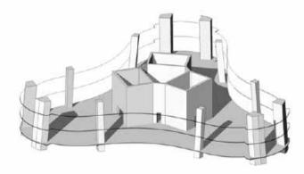
Figure 7. Original Scheme: Larger Core Wall Setback at Level 91 (Source: Thornton Tomasetti)
