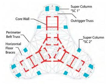
Figure 4. Wuhan Greenland Center Main Tower Structural System (Source: Thornton Tomasetti)
