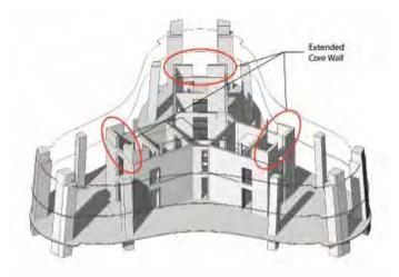
Figure 8. Current Scheme: Less Core Wall Setback at Level 91 (Source: Thornton Tomasetti) 图8. 现行方案: 91层尺寸较小的核心简缩进 (来源: 宋腾添玛沙帝 Thornton Tomasetti
