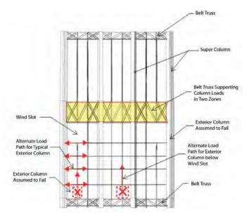
Figure 6. Progressive Collapse Analysis of Exterior Frame (Source: Thornton Tomasetti) 图6. 外部框架抗连续性倒塌分析(来源:宋腾添玛沙帝 Thornton Tomasetti)
