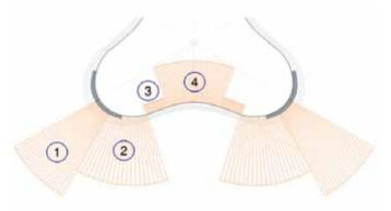
Figure 12. Revised Partial Floor Plan Showing Compound Curve Radii Used (Source: Thornton Tomasetti)
