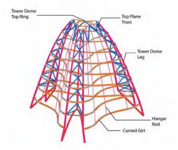
Figure 10. Tower Dome Structure (Source: Thornton Tomasetti) 图10. 塔顶弯拱结构(来源:宋腾添玛沙帝 Thornton Tomasetti)
