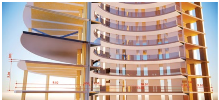
Figure 7. Conceptual partial section. An in-floor steel beam system minimizes the required structural floor assembly heights to 300 mm, resulting in reduced floor-to-floor heights, material volumes, and associated costs.
