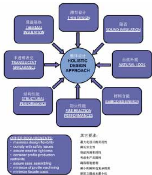
Figure 4. representation of performance requirements set for the TEC façade project. All the requirements have been considered at the same time with a holistic approach (Source: Permasteelisa Group, 2012)
