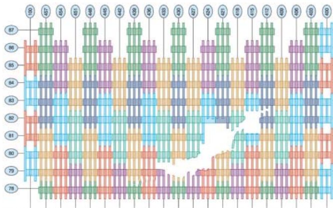
Figure 1. Damage to South Face of WTC 2 © NIST
