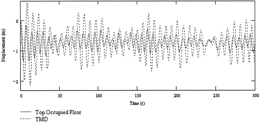
Figure 1 Floor and TMD Motion for an Across-Wind Event.
