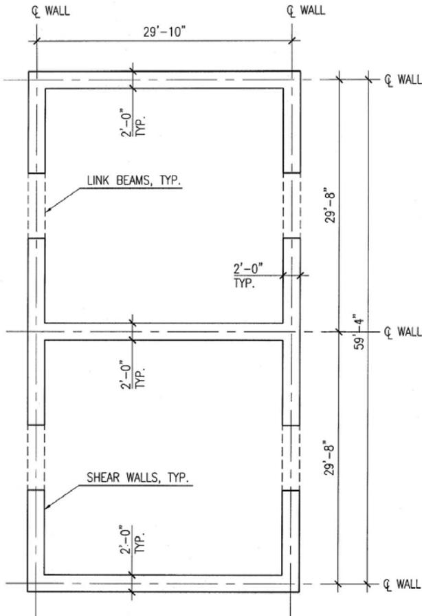
**Figure 1 – Typical Shear Wall Core Plan**
