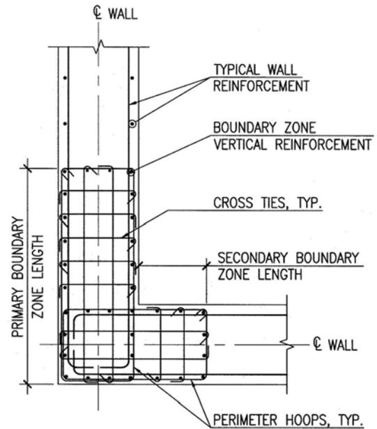
**Figure 5 – Typical Boundary Zone Detail with Conventional Confinement Reinforcement**
