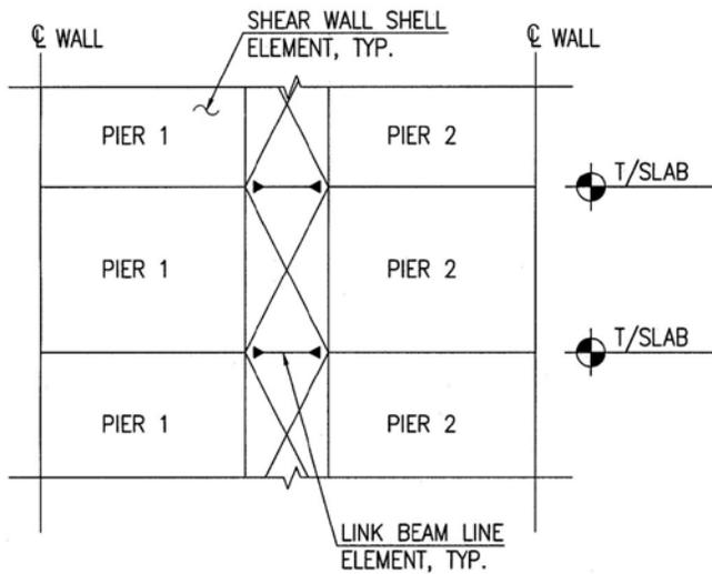
**Figure 4 – Typical Shear Wall Elevation and Pier Assignments**
