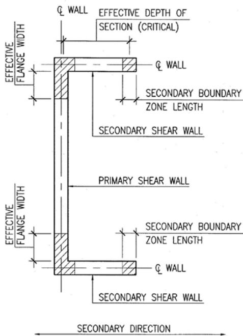
**Figure 3 – Shear Wall “C” Plan Section, Secondary Shear Wall**
