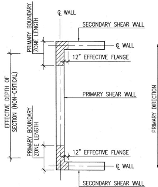
**Figure 2 – Shear Wall “C” Section, Primary Shear Wall Element**
