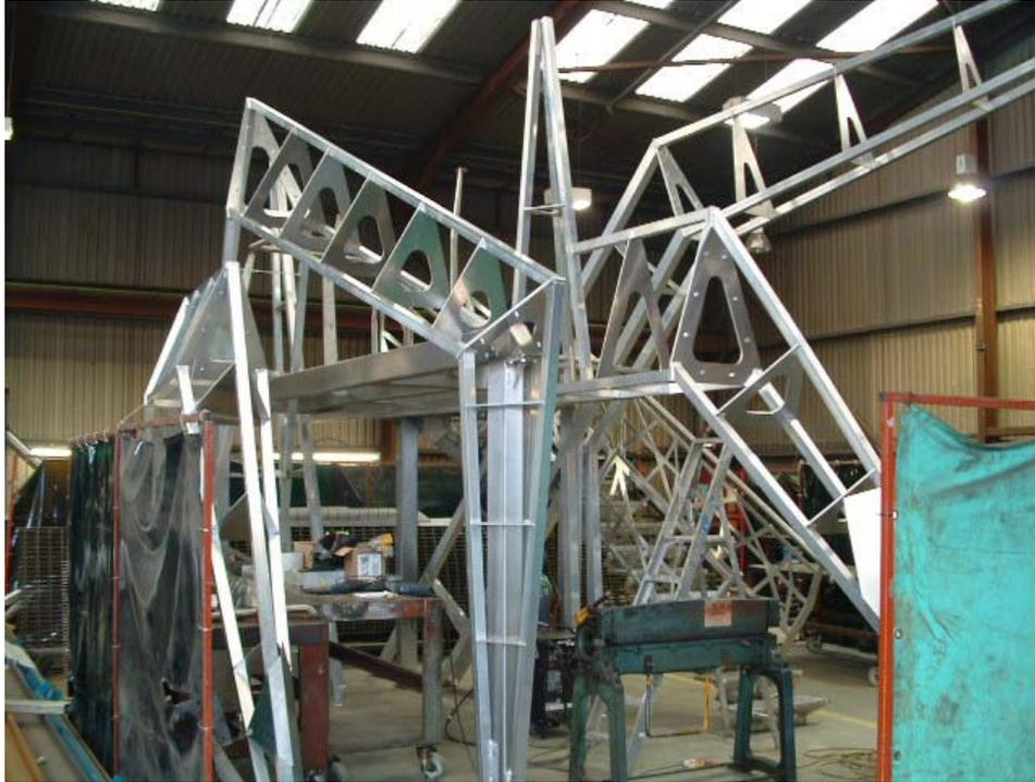
**Figure 4: Fabricating the stand in the factory**
