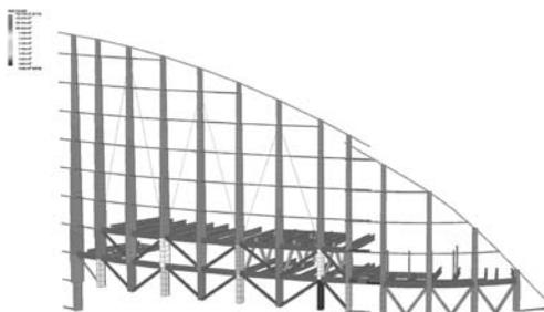
**Figure 26** West sail finite element framing model.
