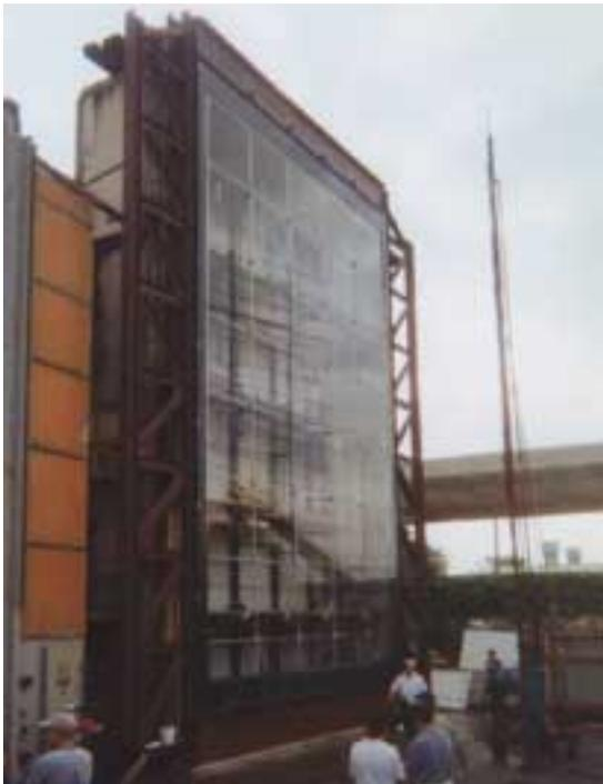
Fig. 5 Mock-up testing a net wall (courtesy of Lohan Associates)
