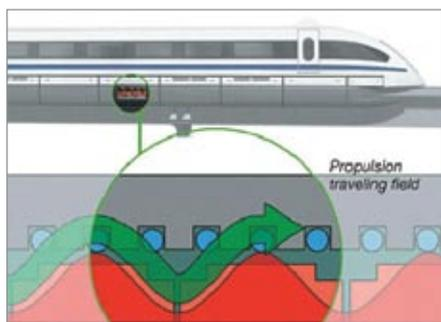
fig 4. Section showing propulsion system for typical mag lev train. Source: Maglev train elevation. [Online Image] Available: [http://www.transrapid.de/cgi-tdb/en/basics.pr?g?session=d82f8833463f50c9&a\\_no=41](http://www.transrapid.de/cgi-tdb/en/basics.pr?g?session=d82f8833463f50c9&a_no=41),
