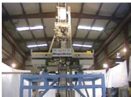
fig 5. MagneMotion's mag lev elevator platform. Source: Advanced weapons elevator demonstration. [Image Clip from Online Video] Video Available <http://www.magenmotion.com/products/elevators/main.shtml>
