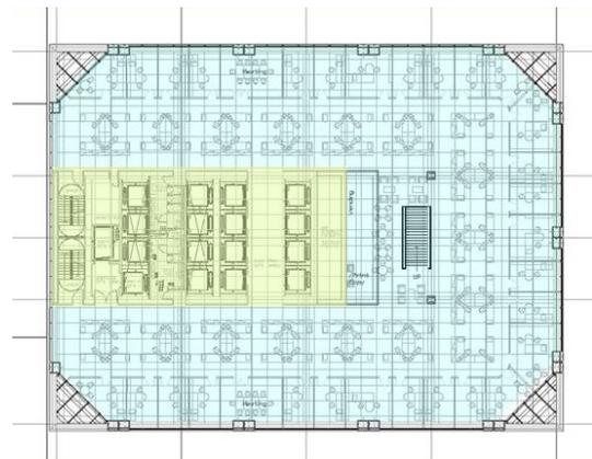
Figure 5. Typical office floor layout
