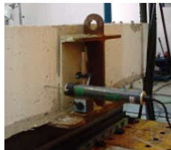
Fig. 9. Measurement of End Slip
