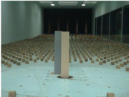
**Fig. 4.** A view of relative building arrangement in the wind tunnel
