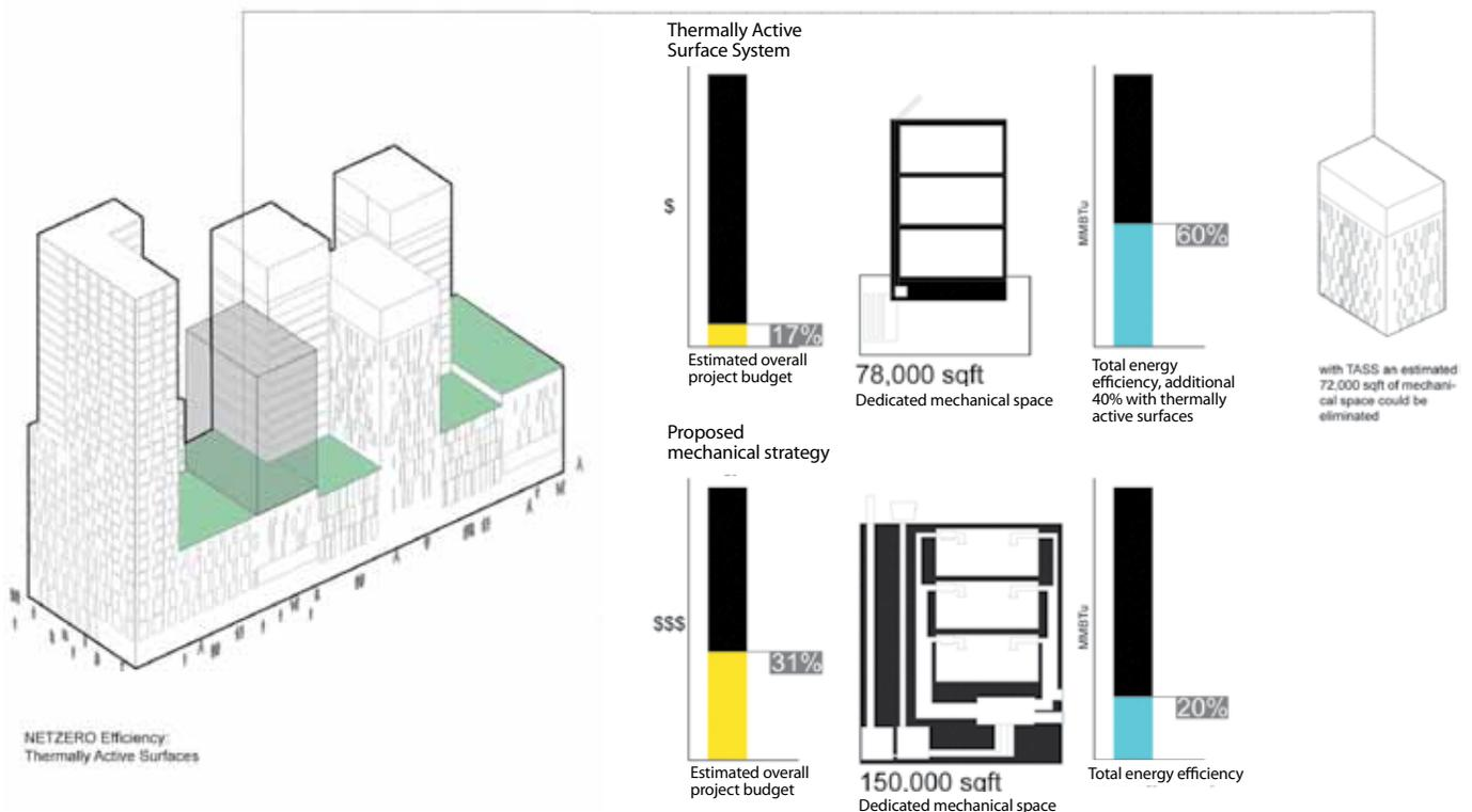
Figure 3. Heating and cooling systems comparison between forced air and Thermally Active Surface System (TASS).
