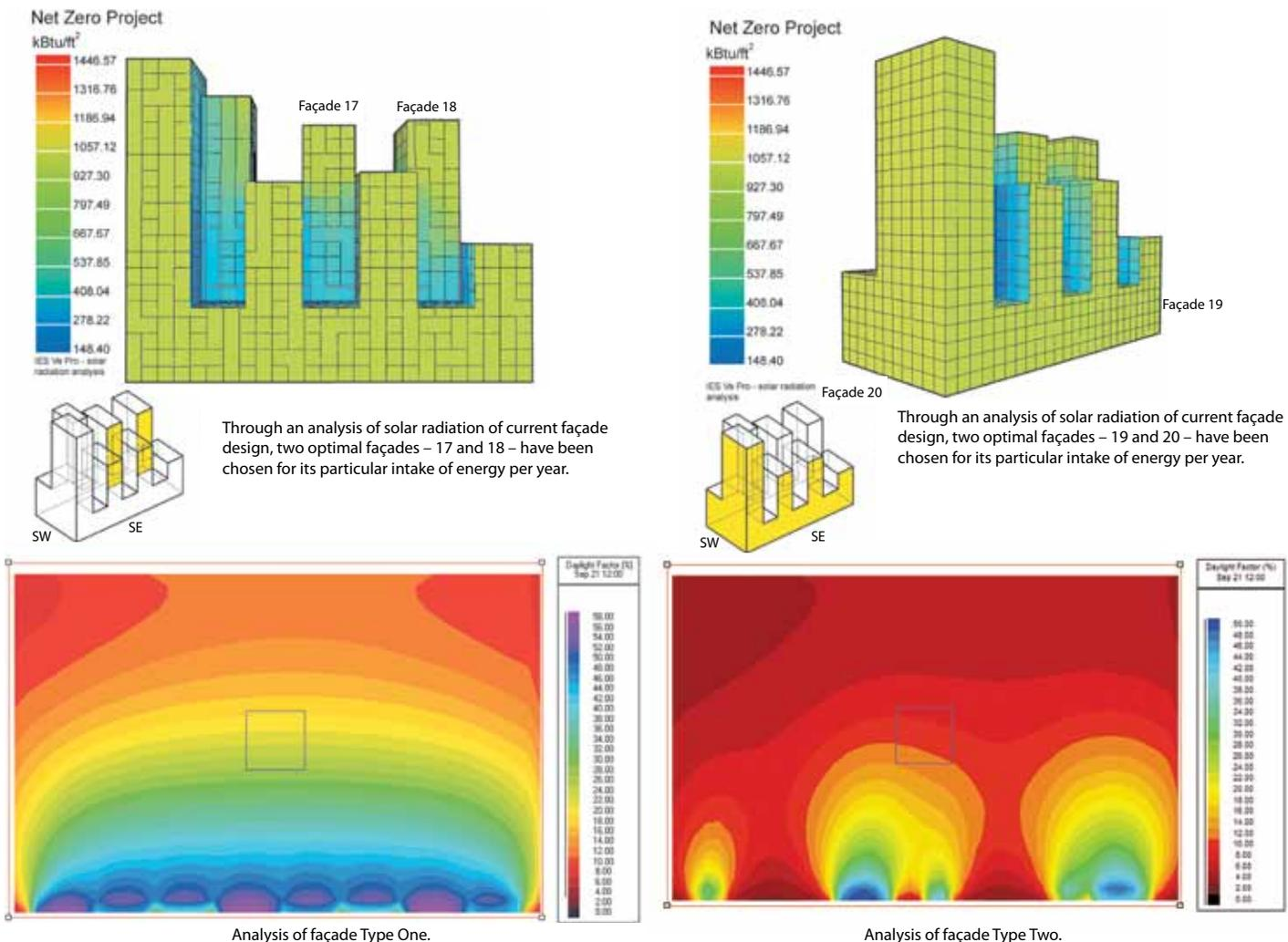
Figure 5. Determining the curtain wall system
