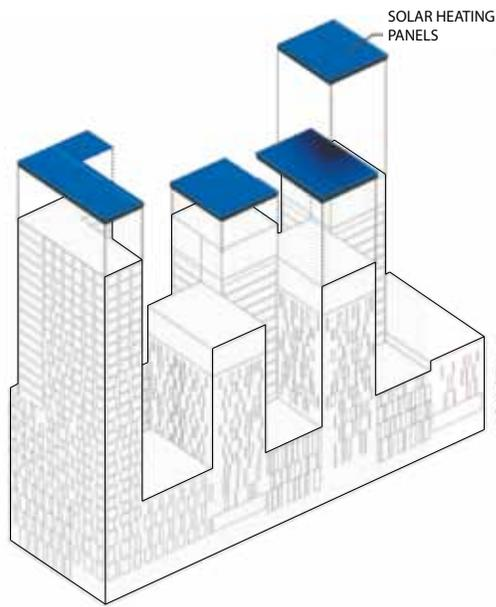
Figure 4. Solar Thermal (ST) panels.
