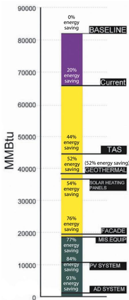
Figure 8. Overall energy footprint after all energy-efficiency options are combined.
