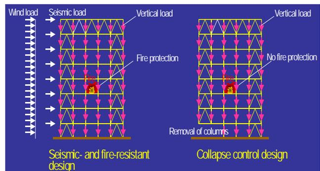
Fig. 2. Image of Collapse Control Design.
