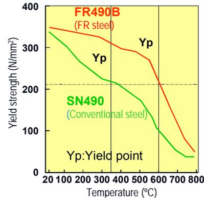
Fig. 9. Transition in Yield Strength of FR Steel and General Steel due to Temperature
