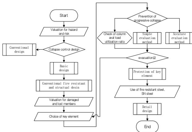
Fig. 3. Outline of Recommended Flow of Collapse Control Design
