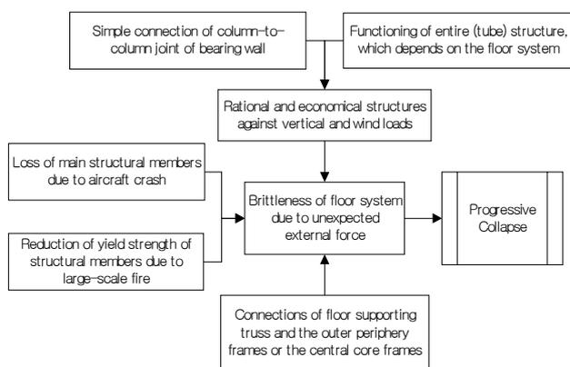
Fig. 1. Analysis of Causes of WTC Collapse.
