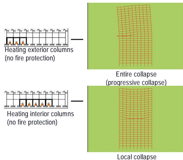
Fig. 6. Analysis Results for Thermal Elasto-Plasticity and Buckling during Fire
