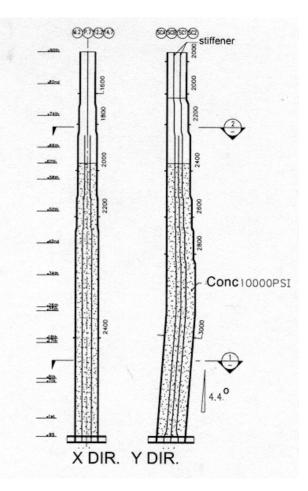
**Fig. 5.** Supercolumns are filled with high-strength concrete for added stiffeness as shown shaded here.
