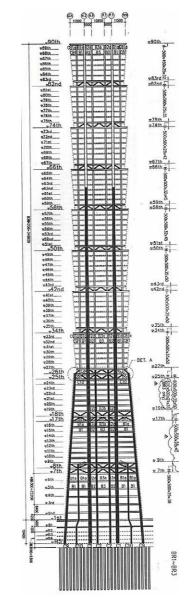
**Fig. 10.** Elevation of a perimeter moment frame line with belt trusses. Shading indicates extent of concrete fill in supercolumns.
