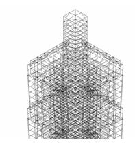
**Fig. 11.** The 3-D computer model for Taipei 101 shows core bracing, perimeter moment frames and vertical and horizontal trussing at module setbacks every 8th floor.
