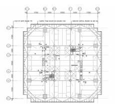
**Fig. 4.** This typical setback floor plan shows sawtooth corners, a braced core with 16 steel box columns, outriggers to eight perimeter concrete-filled steel box supercolumns, upper (inner) and lower (outer) perimeter wideflange moment frame columns and in-floor bracing to transfer story shear between modules.
