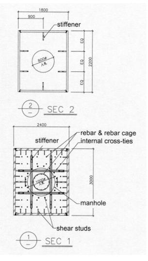
**Fig. 7.** Supercolumn box plan details show stiffeners, diaphragms, shear studs and cross-box ties.
