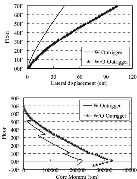
**Fig. 8.** Effect of the Outrigger
