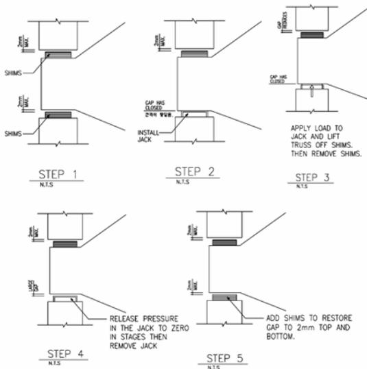
Fig. 15. Sequential Adjustment Steps
