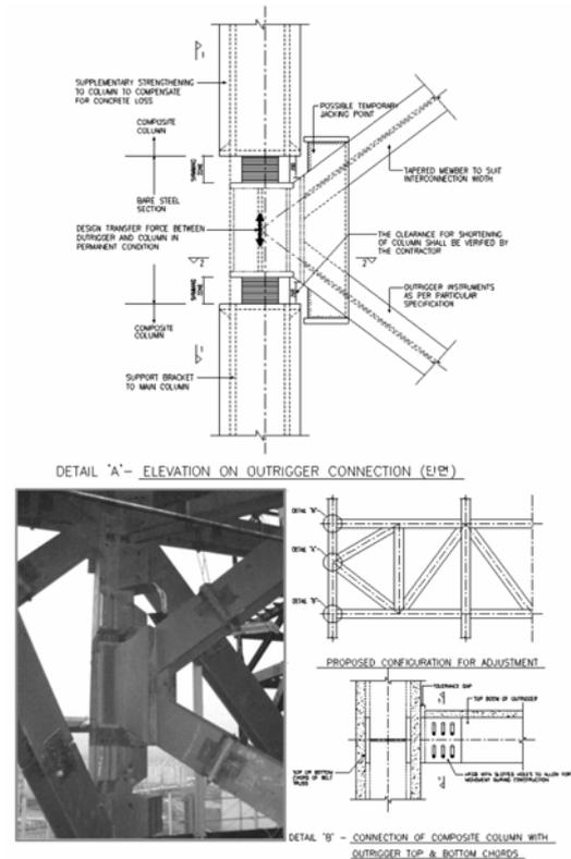
**Fig. 14.** Connection Details for Outrigger Adjustment
