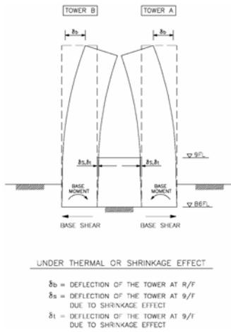
Fig. 4. Thermal Movement and Shrinkage
