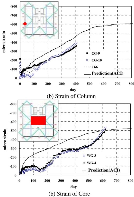
Fig. 12. Axial strain (Prediction & Measurement)
