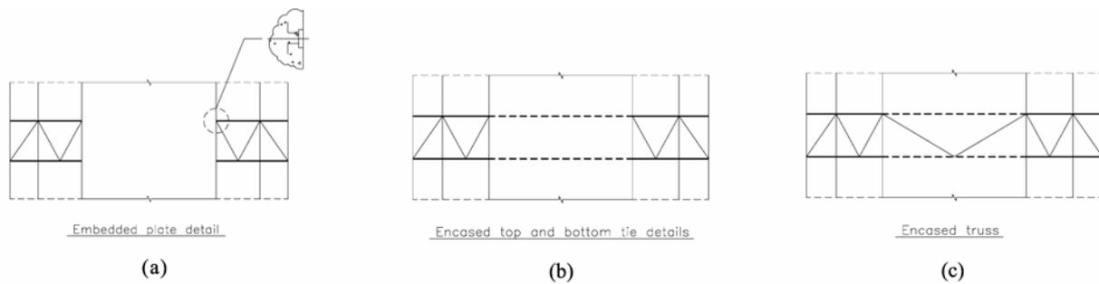
**Fig. 13.** Connection between Outrigger and Shear Wall
