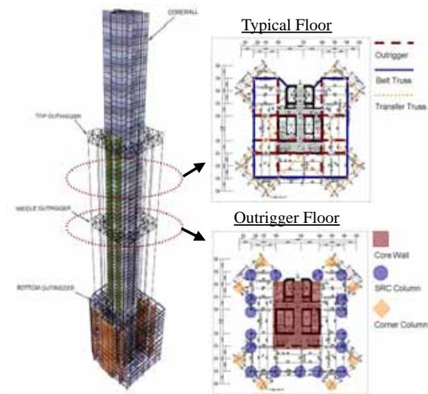
Fig. 2. Framing Plan of Tower
