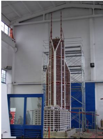
Fig. 3. Structural Model in SKLDRCE.
