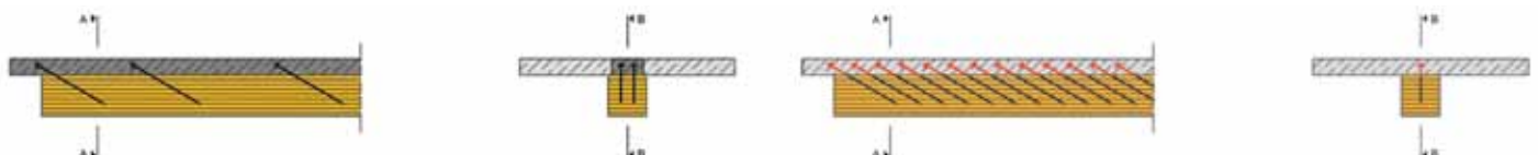
Figure 9. Würth connector – certified connecting system with plastic and/or steel washers as anchors embedded in concrete and screwed into the timber beams.
