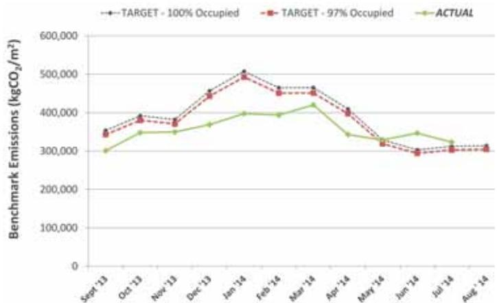
Figure 6. Actual monthly benchmark emissions vs. simulated NABERS benchmark emissions.
