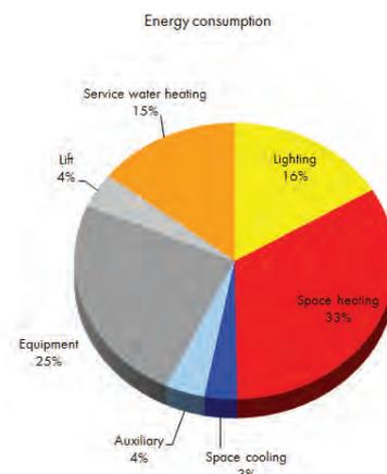
Figure 3. Distribution of energy consumption in Plot 15. (Source: Werner Sobek, Stuttgart)
