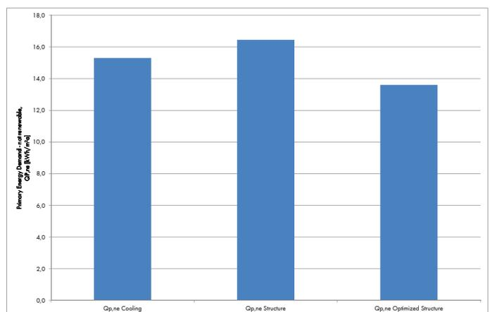
Figure 5. Comparison of average energy consumption for cooling and structure per year. (Source: Werner Sobek, Stuttgart)
