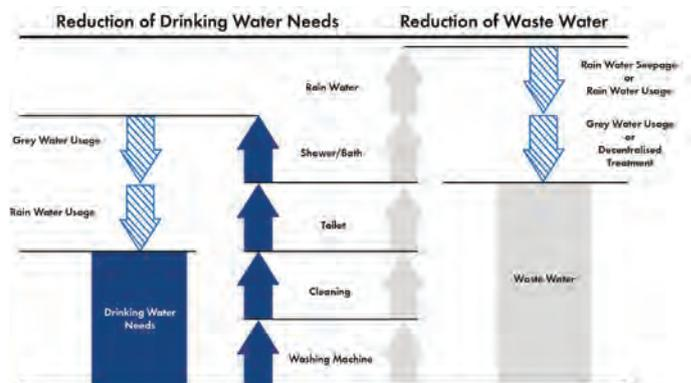
Figure 2. Reduction of water consumption in Plot 15. (Source: Werner Sobek, Stuttgart)
