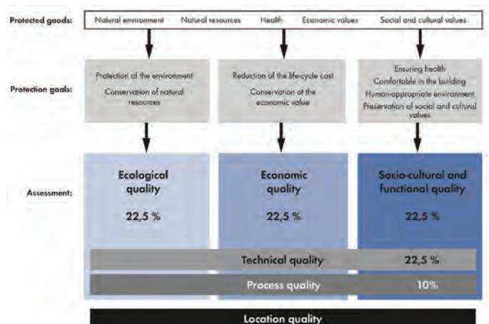
Figure 4. Basic structure of the DGNB rating tool. (Source: Werner Sobek, Stuttgart)
