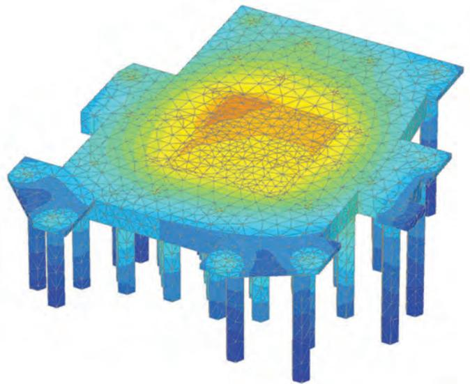
Figure 3. Analysis Model of Foundation
