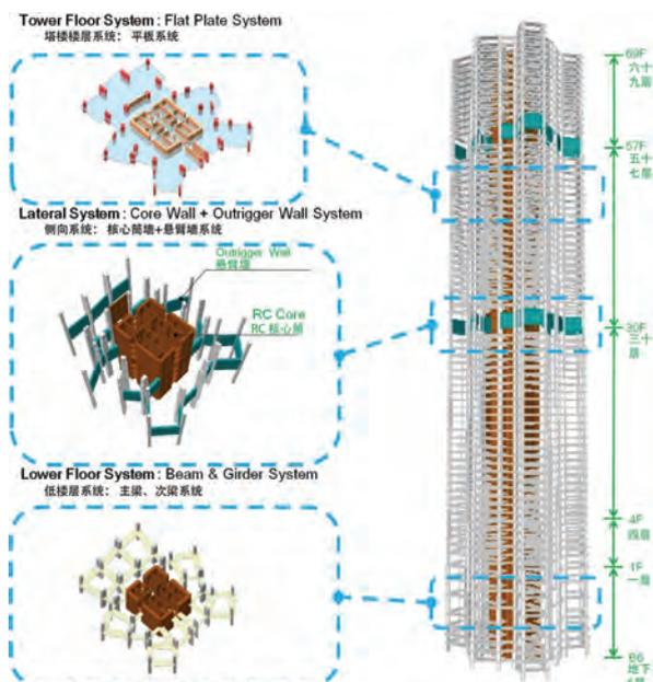
Figure 2. Tower Structural System.
