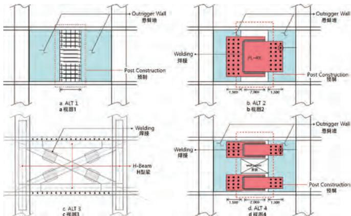
Figure 6. Alternative of Delay Joint of Outrigger Wall For Construction
