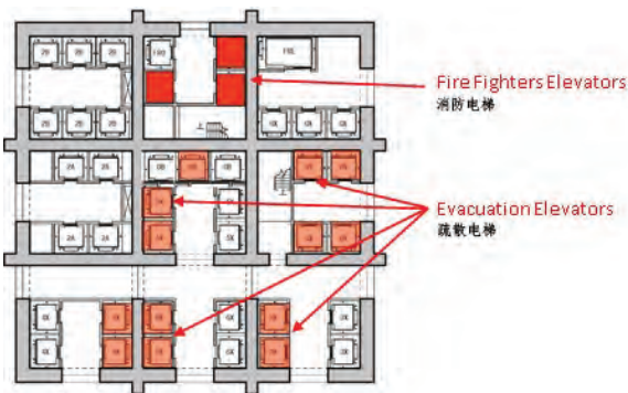
Figure 8. Using elevators in evacuation. (Source: Floor plan courtesy of Gensler; Modeling courtesy of Rolf Jensen & Associates, Inc.)
