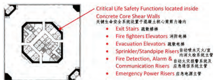
Figure 4. Critical Life Safety Systems. (Source: Floor plan courtesy of Kohn Pedersen Fox Associates; Modeling courtesy of Rolf Jensen & Associates, Inc.) 图4 关键的生命安全系统 (来源: Kohn Pedersen Fox Associates 友情提供的平面图; Rolf Jensen & Associates, Inc 友情提供的模型)
