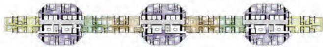
Figure 7. Sunrise: The typical floor plan delivers a high density layout with a high proportion of truly dual and triple aspect residences that do not overlook 图7.日出:典型户型图提供了一个高密度的布局,同时大部分住宅拥有双面、三面采光,且不产生对视
