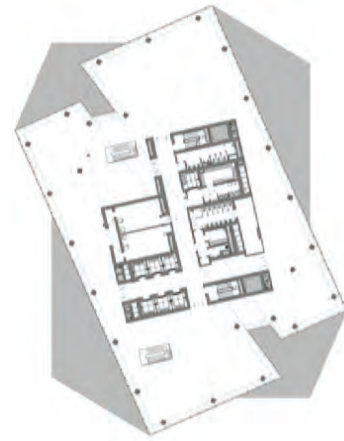
Figure 9. Sarona Tower: The Floor Plan Evolves Geometrically (Source: Moshe Zur Architects Urbanists /with Architect David Azrieli)
