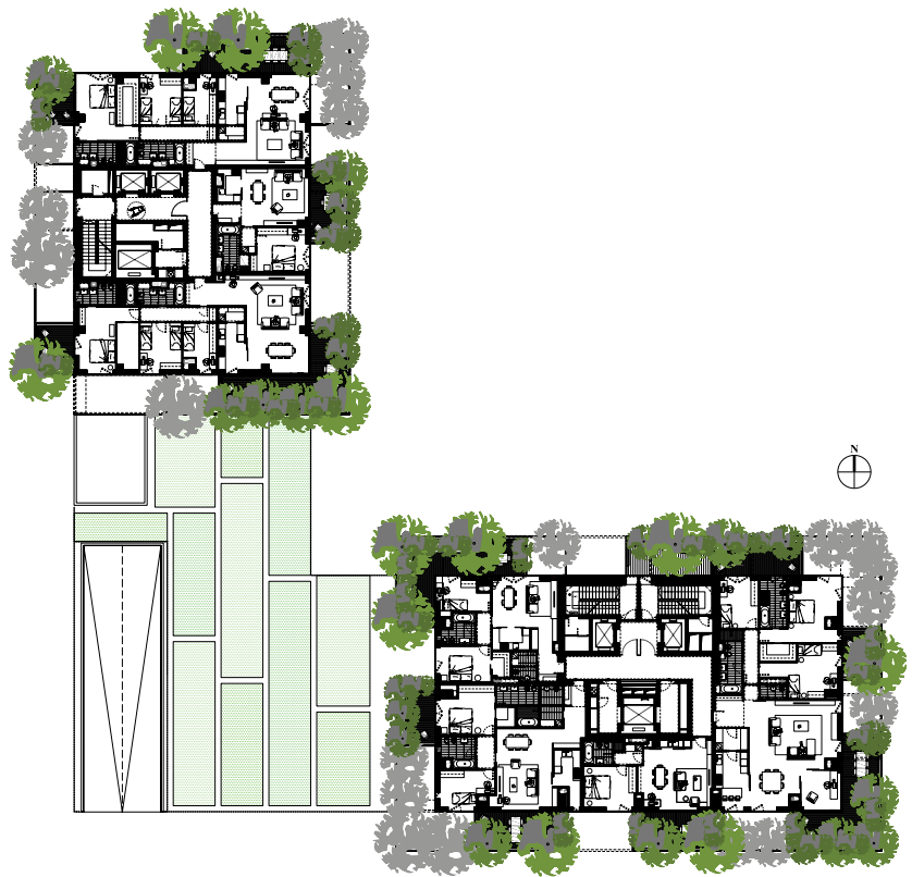
Figure 5. Typical plan showing the terraces cantilevered from the main tower plans. © Stefano Boeri Architetti
