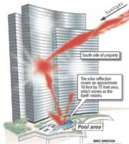
Figure 4. The solar reflection cast during the day from the Vdara Hotel, Las Vegas. Source: Las Vegas Review Journal
