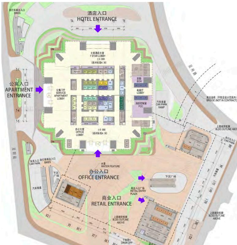
Figure 2.4. Site access diagram (Source: Gensler)
