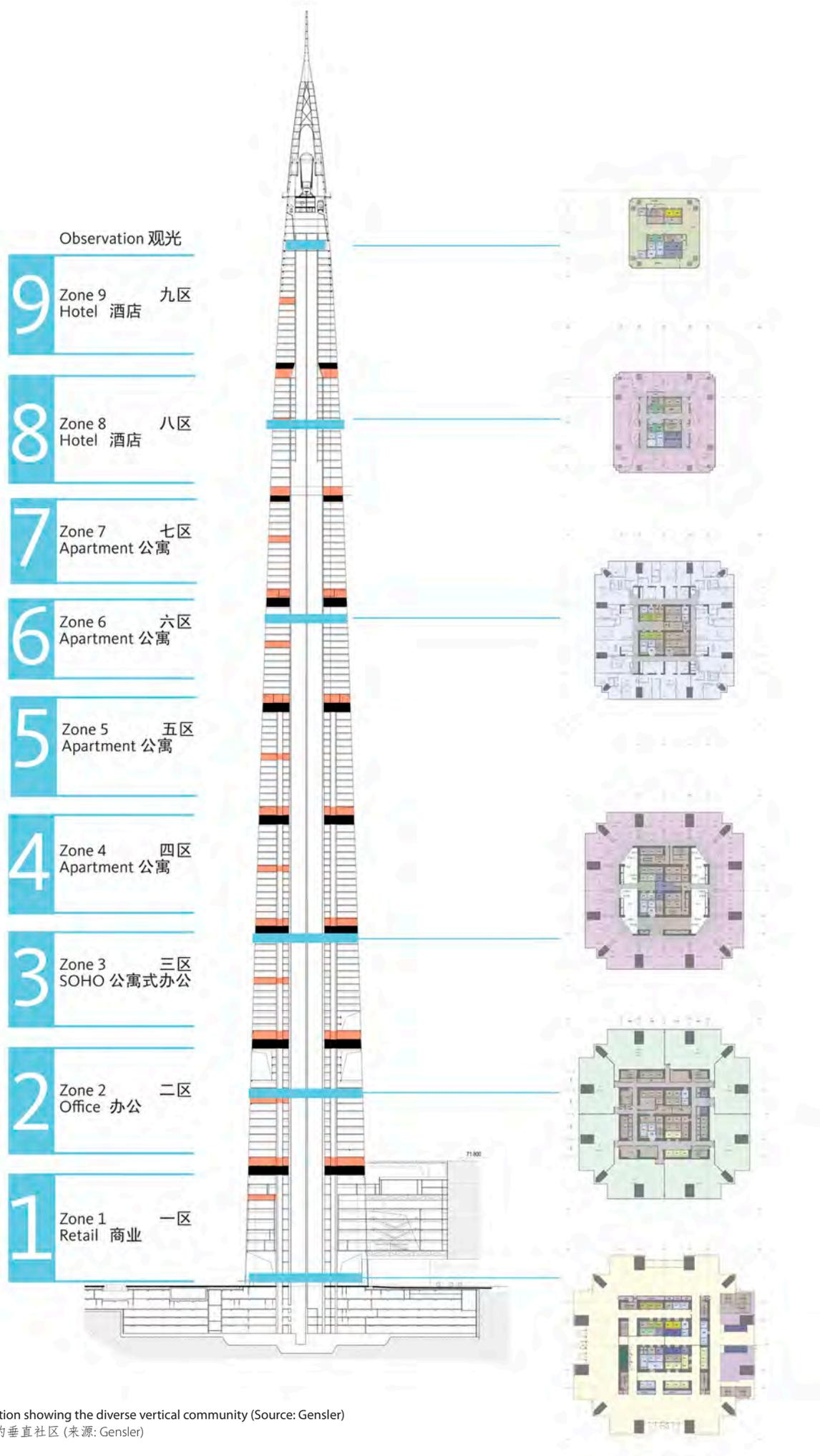
Figure 2.3. Section showing the diverse vertical community (Source: Gensler)
