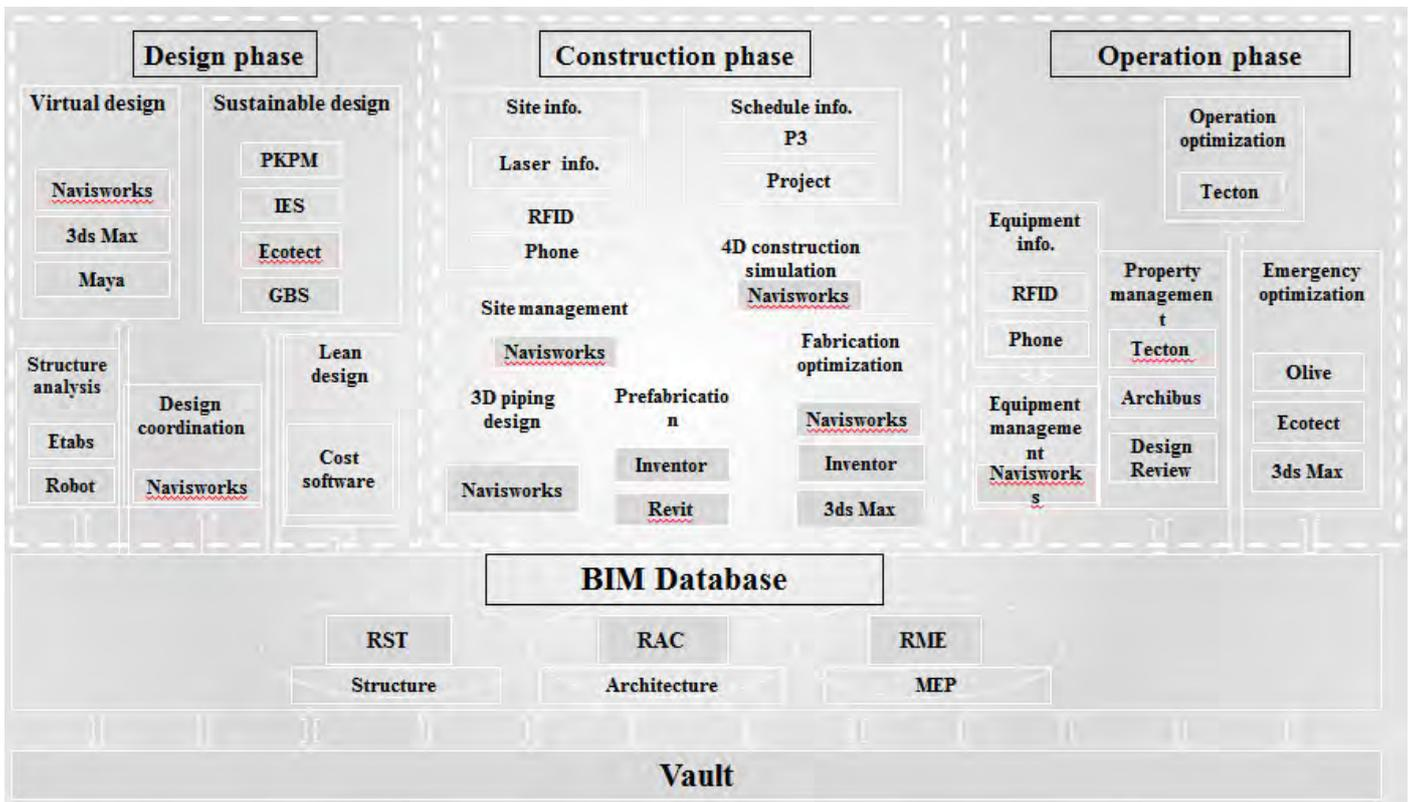
Figure 5.4. BIM technical framework (2010 version) (Source: Shanghai Tower Construction & Development Co., Ltd)
