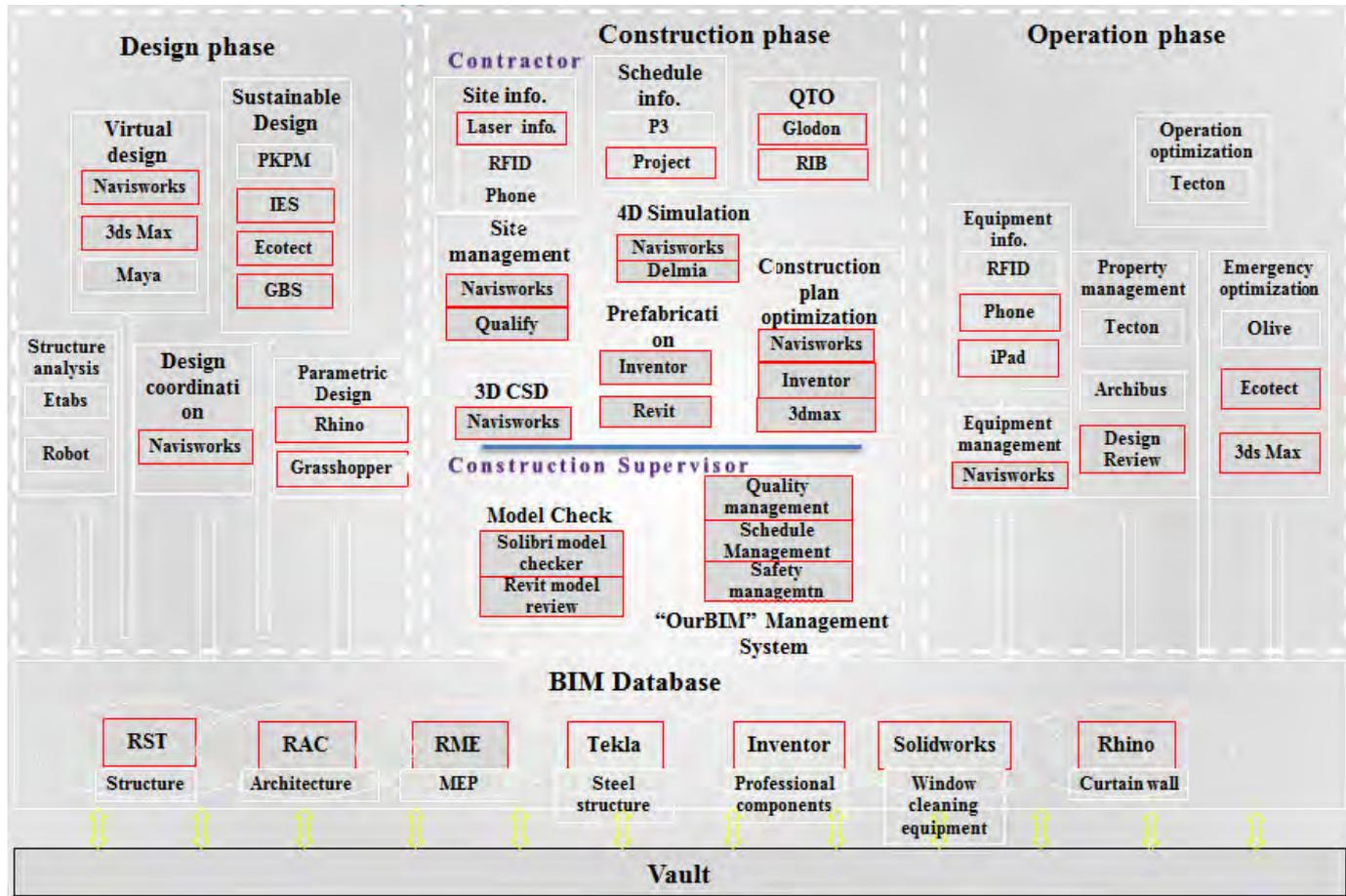
Figure 5.5. BIM technical framework (2013 version) (Source: Shanghai Tower Construction & Development Co., Ltd)
