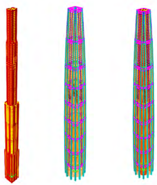
Figure 3.33. Structural lateral system of Zhongnan Center (Source: Guangjing Sha) 图3.33. 结构抗侧力体系 (来源: 沙广璟)
