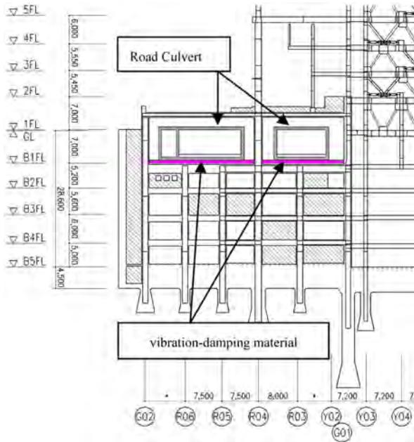
Figure 7. Road Culvert Structure and Underground Building Structure.
