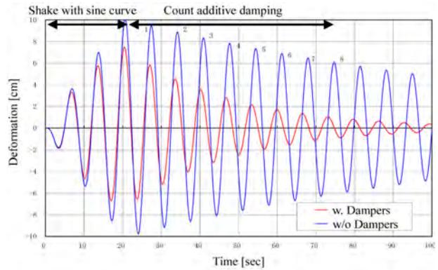
Figure 9. Results of the free vibration response.
