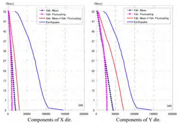
Figure 10. Story shear force by wind load. [Maximum for Y dir. 35°].
