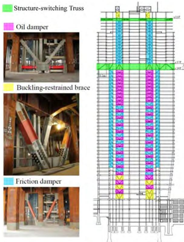
Figure 3. Arrangement of Response-control Devices and Structure-switching Truss.
