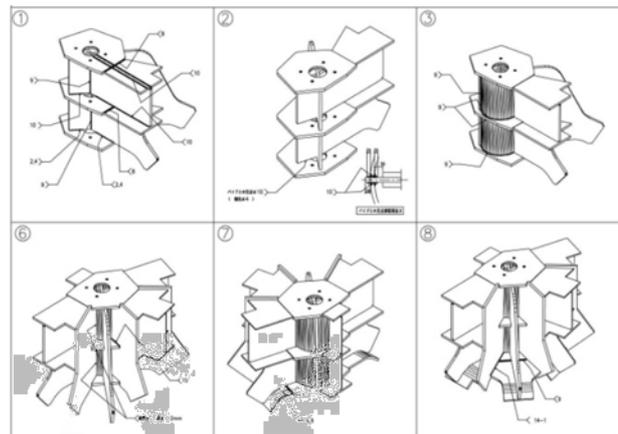
**Figure 5.** Column connection.
