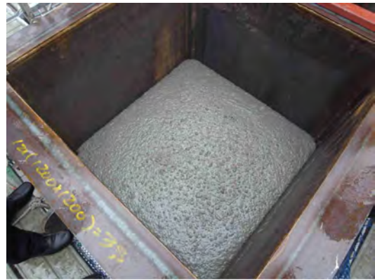
Figure 17. Concrete filling confirmation test.
