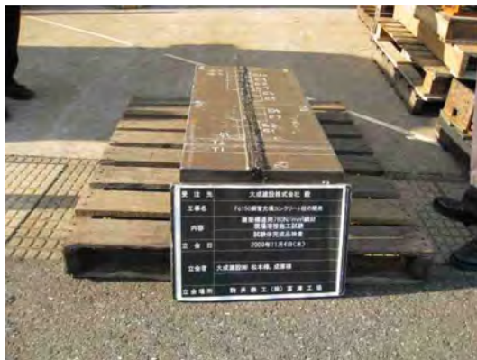
Figure 19. Site weld construction test piece.
