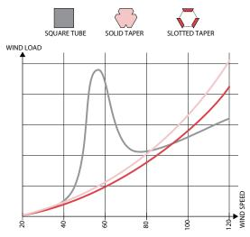
Figure 10. Wind response of three primary tower types. © RWDI
