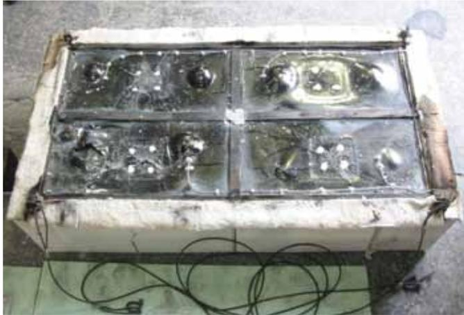
Figure 8. Test specimen after heating (two upper layers were removed to confirm no cracking in the third layer of the glass laminates).
