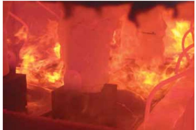
Figure 9. Test specimen during heating (from observation window of test furnace).
