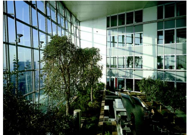
Figure 7. The 1997 Commerzbank in Frankfurt is still one of the best examples of significant, communal skygardens in a tall building anywhere in the world. This office building is also potentially an excellent model for an idealized residential building, with thin, cross-ventilated floors of apartments all grouped around one of ten “gardens in the sky,” where a sense of residential community can develop. Copyright: Nigel Young - Foster + Partners.
