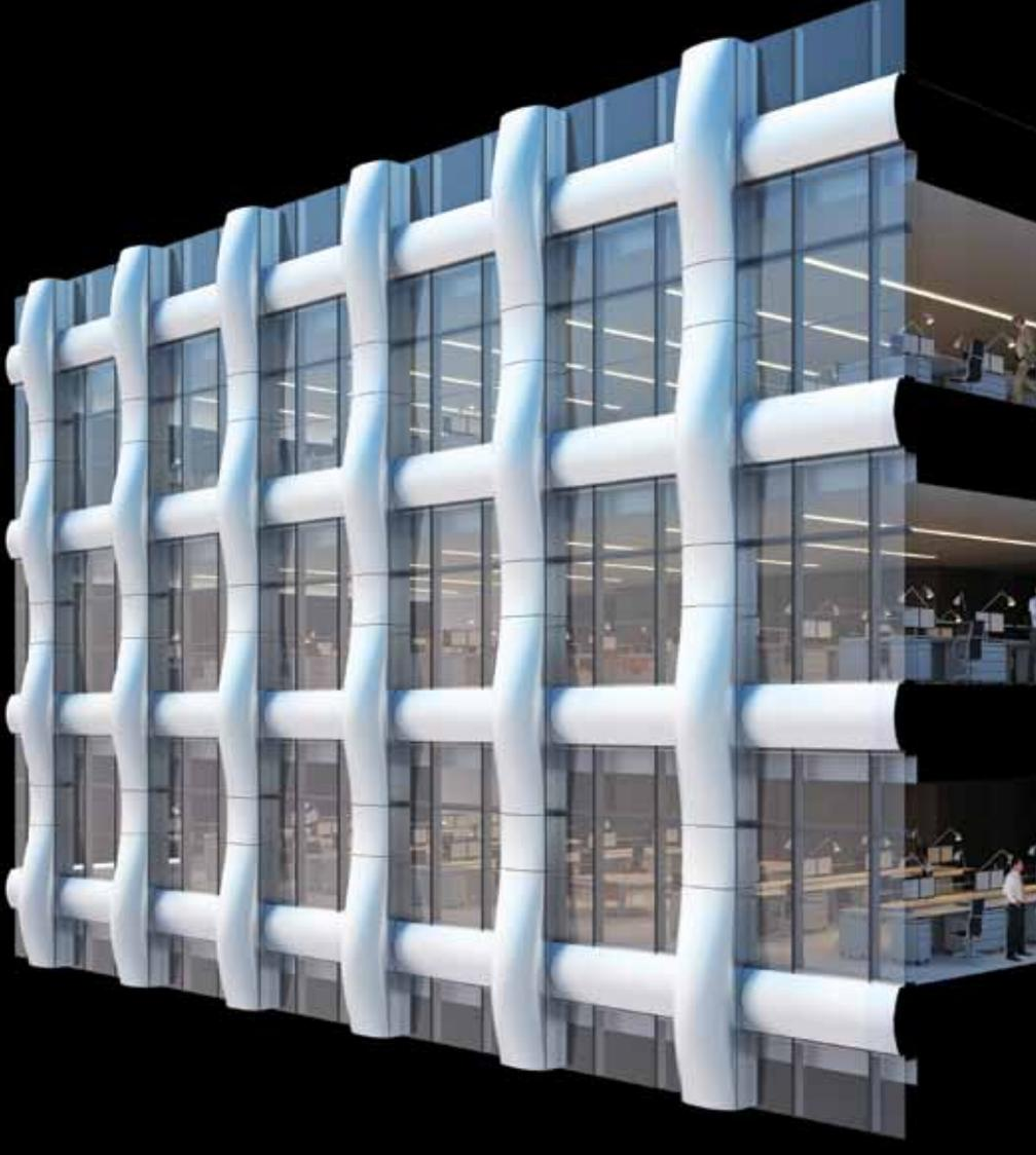
Left: Façade rendering showing inset glass panels, and sculptural metal column covers that double as shading fins. Source: Skidmore, Owings & Merrill
