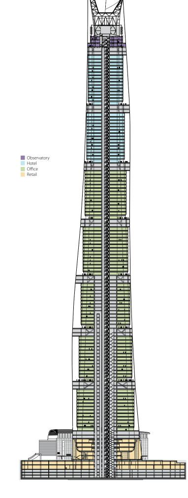
"Shanghai Tower provides a vision of vertically integrated space through the signature design of a double façade that creates unique sky lobbies, filled with vegetation, offering the potential for socializing, and providing relief from the isolative nature of tall buildings without the necessity of descending to the ground."
