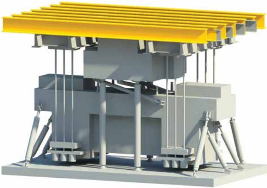
Figure 7. Damper (Source: DeSimone Consulting Engineers, PLLC)
