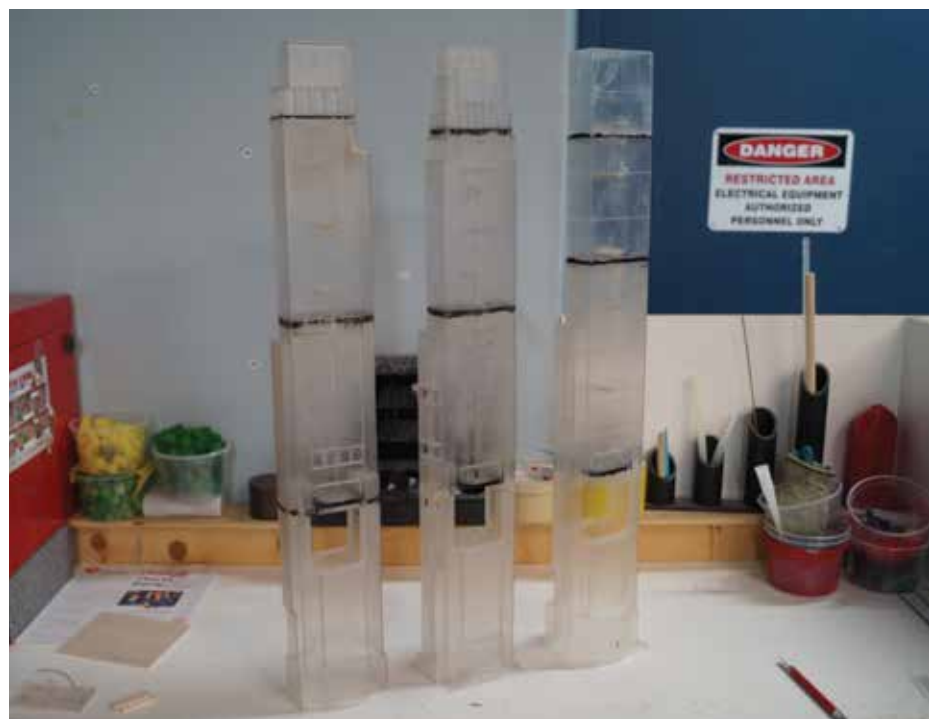
Figure 1. Tower Massing Options for Testing (Source: DeSimone Consulting Engineers, PLLC)
