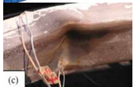
Figure 9. Nonlinear simulation of hinge formation and plastic strain development on 3-story brace on Reforma 509. Test photo from Fell (2008). (Source: Arup)
