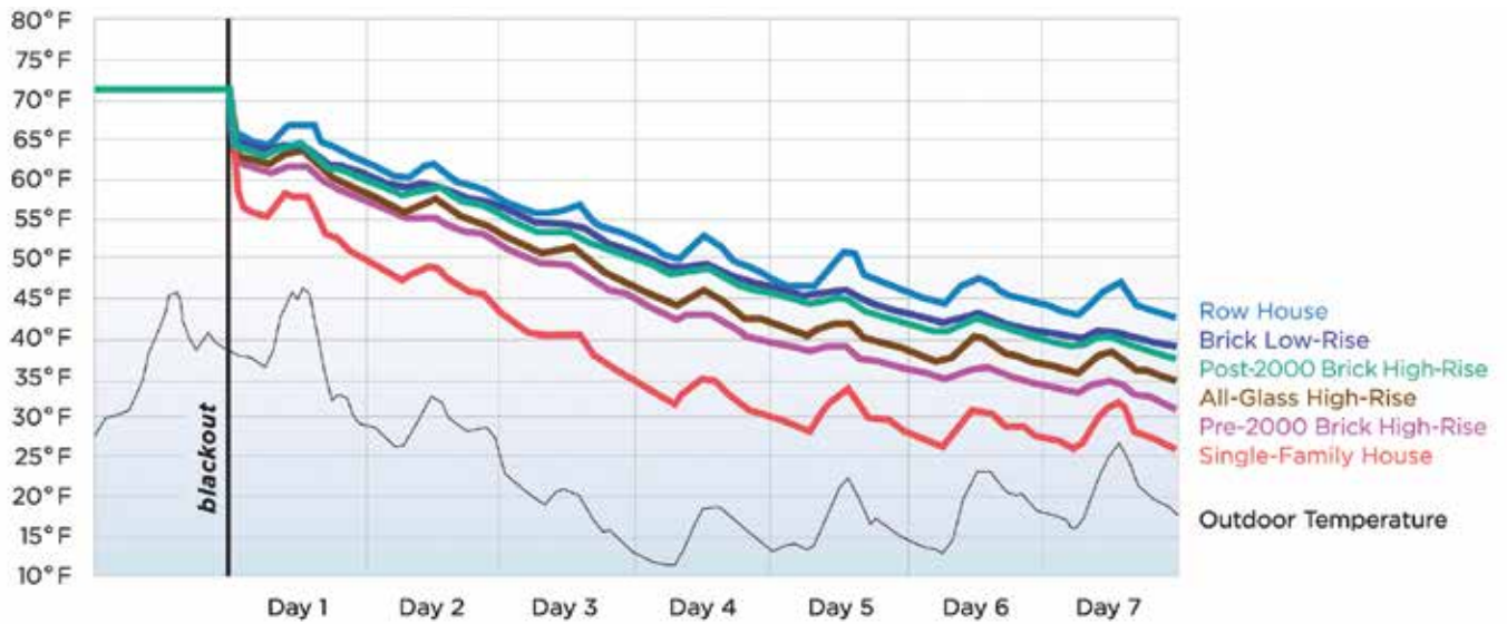
Figure 7. Typical Building Indoor Temperatures During a Winter Blackout (Source: Urban Green Council)
