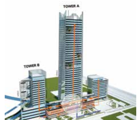
Figure 6. Vertical and horizontal connectivity through the Telkom campus. Towers A and B are connected to the existing building on site through a common podium structure. (Source: Woods Bagot)
