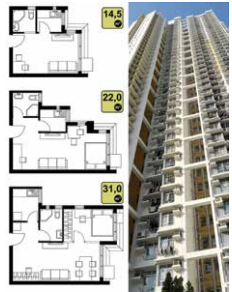
Figure 11. Modular Flat Design. Choi Tak Estate, Hong Kong (Photo source: Elena Generalova, floor plan source: http://www.legco.gov.hk/yr12-13/english/panels/hg/papers/hg0702cb1-1391-1-e.pdf )
