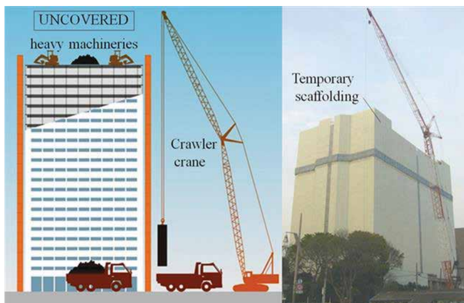
Figure 1. Conventional demolition method in Japan (Source: Taisei Corporation)
