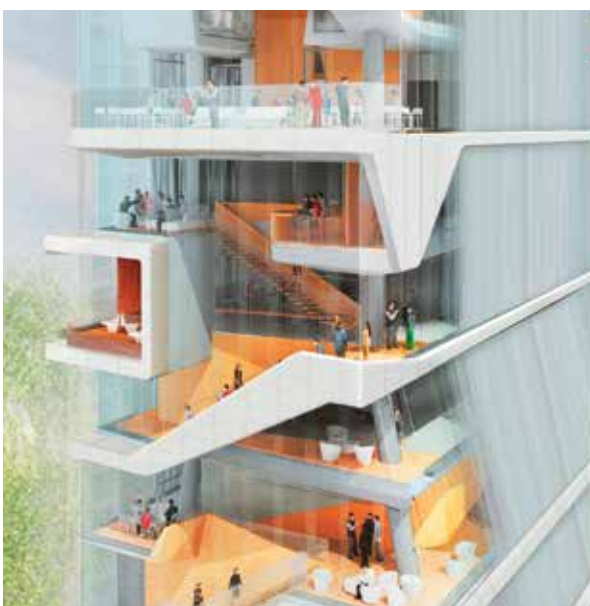
Figure 9. The cantilevered slab performance was coordinated by "neighborhood", here in Floors 7 through 10, with the façade system requirements during a design assist process with the Curtain Wall Contractor (Source: Diller Scofidio + Renfro left / Leslie E. Robertson Associates)
