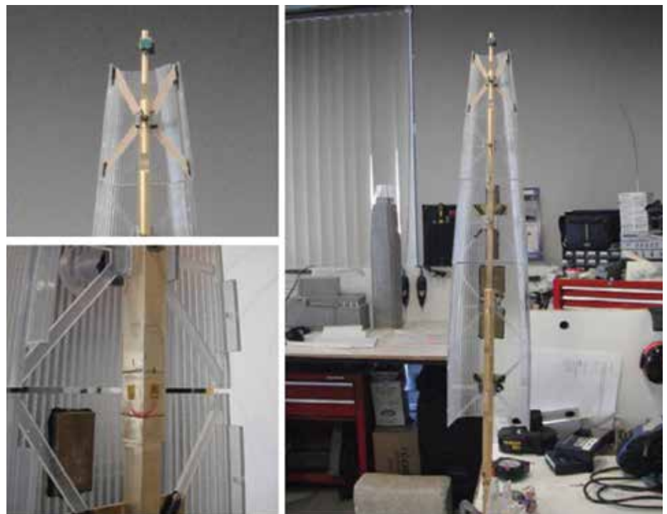
Figure 6. Aeroelastic model (Source: Chang Minwoo Structural Consultants)
