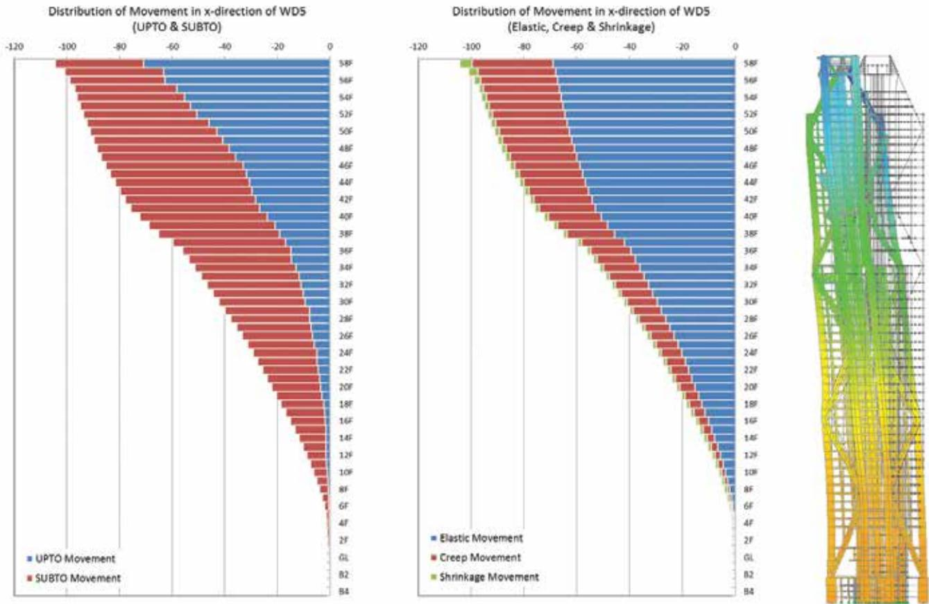
Figure 7. Results of construction stage analysis of the Tower regarding deviation from verticality (Source: Daewoo E&C)
