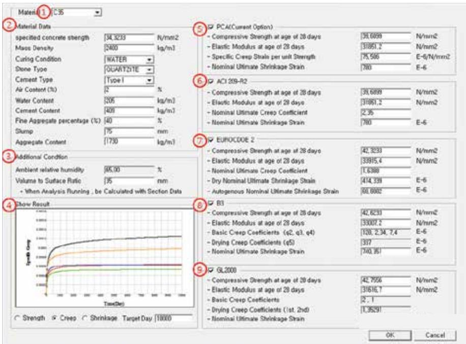
Figure 9. Input window for time-dependent properties of concrete in ASAP (Source: Daewoo E&C)
