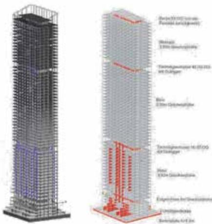
Figure 6. Load Transfer from the Core to the Columns (Source: Bollinger + Grohmann)
